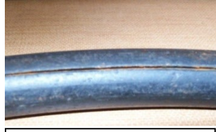
Failed pipe seam covered under warranty
