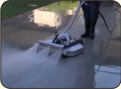
Caster pivot lock allows the operator to choose to lock casters for use in straight lines or unlock for cleaning side-to-side.
