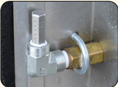
The under-deck spot remover uses a "six-shooter" nozzle to blast away gum or paint.
