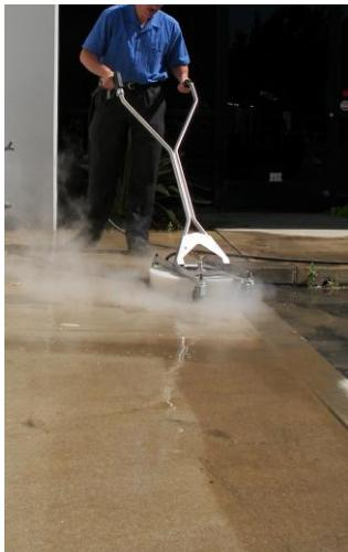
The Hydro Twister® is a flat surface cleaner that connects to a pressure washer and uses a spray bar rotating at a high speed within 1" of the ground. It will clean concrete more consistent than an operator with a spray wand, with less fatigue, and 10-20 times faster. Simply move the twister over the surface and watch a clean path appear behind the unit.
