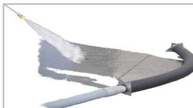
berms to divert wash water away from storm drains and toward a vacuum pickup device. The vacuum system can be used to
