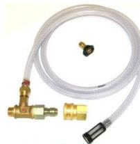
An optional DOWNSTREAM INJECTOR is available if harsh chemicals need to be applied. The downstream injector will apply chemicals only at low pressure, by installing black soap nozzle or opening spray wand valve if equipped. If equipped standard with downstream injection, adjust concentration level by turning brass collar on the injector, or the knob on pump or control panel. Read and follow all safety instructions on the detergent label.
