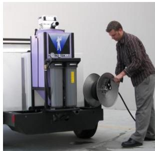
**HOSE REELS:** Hose reels are available for convenient and quick storage of both discharge and inlet hoses. Different hose reels options are available for trailer mounting, machine mounting, or as base
