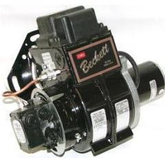
**DIESEL FIRED BURNER:** The diesel-fired burner is a forced draft pressure-atomizing burner. Diesel fuel is sprayed out of an atomizing nozzle, mixed with air, and ignited by a high voltage spark. The flame is directed towards the coils of pipe, which in turn, heats the water flowing through it. Use clean #2 DIESEL FUEL for the burner or substitute #1 diesel, light fuel oil, or Kerosene if diesel is not available.
