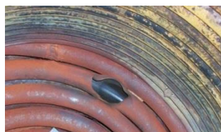
Pipe rupture due to freezing or obstruction
