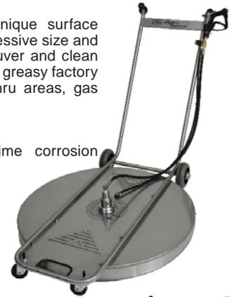
The Hydro Twister ANT20 and ANT28 are surface cleaners that connect to a pressure washer and uses two nozzles rotating at a high RPM within 1" of the ground. It will clean concrete at up to 15 times the speed of an operator using a wand and with more consistency and less operator fatigue. Simply move the twister over the surface and watch a clean path appear behind the unit.
