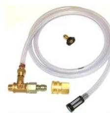
available if harsh chemicals need to be applied. The downstream injector will apply chemicals only at low pressure, by installing black soap nozzle or opening spray wand valve if equipped. If equipped standard with downstream injection, adjust concentration level by turning brass collar on the injector, or the knob on pump or control panel. Read and follow all safety instructions on the detergent label.
