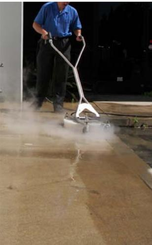
The Hydro Twister® is a flat surface cleaner that connects to a pressure washer and uses a spray bar rotating at a high speed within 1" of the ground. It will clean concrete more consistent than an operator with a spray wand, with less fatigue, and 10-20 times faster. Simply move the twister over the surface and watch a clean path appear behind the unit.
