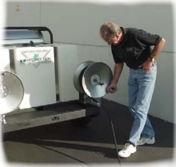
**HOSE REELS:** Hose reels are available for convenient and quick storage of both discharge and inlet hoses. Different hose reel options are available for trailer mounting, machine mounting, or as base mount options. To
