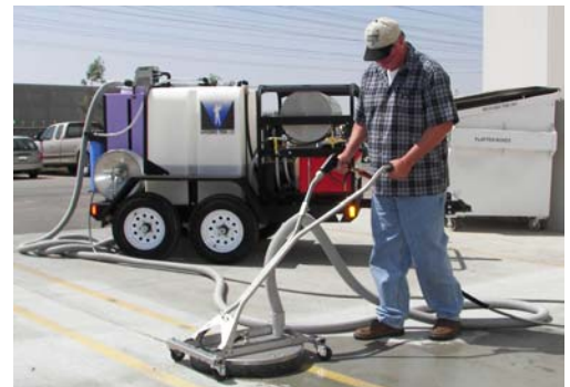
Concrete cleaning & washing with Vac Twister & water recovery
